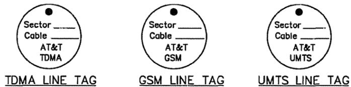
TO PROVIDE ADDITIONAL IDENTIFICATION EACH RF CABLE SHALL BE IDENTIFIED WITH A METAL TAG MADE OF STAINLESS STEEL OR BRASS AND STAMPED WITH THE SECTOR, CABLE NUMBER, AND "AT&T" TO IDENTIFY AT&T MOBILITY CABLES. THE ID MARKING LOCATIONS SHOULD BE AS PER "CABLE MARKING LOCATIONS TABLE". THE TAG SHOULD BE ATTACHED WITH CORROSION PROOF WIRE AROUND THE CABLE. PREFERRED TAG LABELING SHOULD BE AS SHOWN ABOVE "TDMA LINE TAG", "GSM LINE TAG" AND "UMTS LINE TAG".
